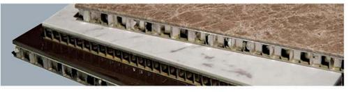
The demand for large yet lightweight stone slabs has led to the development of panels made from thin natural stone sheets (minimum 5 mm thick), bonded to honeycomb panels with epoxy adhesives.
