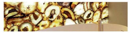
Backlighting is a high-impact use of natural stone, leveraging its translucency — especially that of onyx — with the placement of light sources behind the material to create stunning effects.
